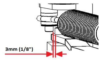
Approximate gap between the base of the main shaft pin and the drive pin viewed from behind the machine.
