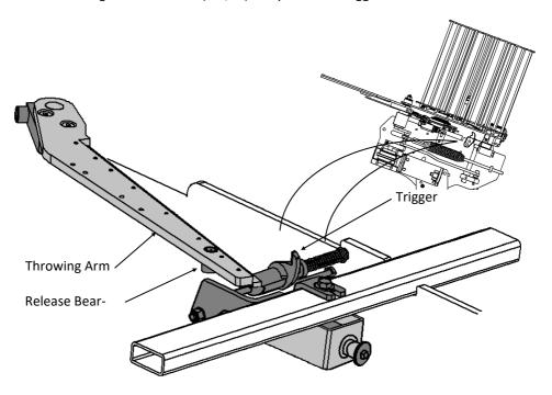
As the arm reaches TDC, the spring is at its maximum. As the arm then passes over TDC the spring takes over and pulls the arm around until it comes to rest with a clunk against the trigger and can go no further. The trigger holds the arm in the cocked position waiting to be fired.
