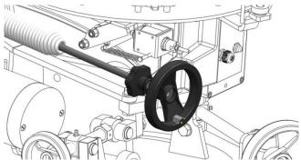
Slacken the smaller of the two hand-wheels on the main spring. Turn the larger hand-wheel as necessary to adjust the tension in the mainspring. This will affect the speed and distance that the clay travels. Lock down the mainspring by retightening the smaller hand-wheel.
