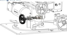
Turn the small hand-wheel located to the left of the machine. Clockwise will tilt the machine to the right, anti-clockwise, to the left.
