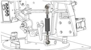
Turn the vertical turnbuckle located towards the front right hand side of the machine. Turning it anti-clockwise with increase the elevation, clockwise will reduce it.
