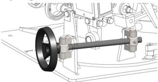
Turn the large hand-wheel at the rear of the machine to change the direction of flight. Approximate angles are marked on the base plate, 'H' denotes the High house, 'L' is the Low house. This will be set approximately at the factory.
